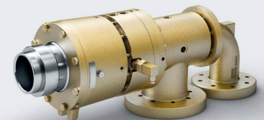
Rotary joints for hot water and steam at high pressures and speeds. Balanced mechanical seal with external water cooling. Meet the special requirements of paper and nonwoven calenders, fiber and corrugated paper plants. Suitable for big, steam-heated dryers. Patented system.
