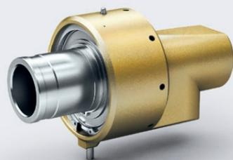
All-purpose rotary joints for water, equipped with mechanical seal and roller bearings. DXS with extremely resistant, ceramic-coated sealing face for higher temperatures and speeds and a long service life.
