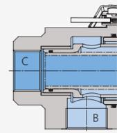
Housing connection B radial - Housing connection C axial
