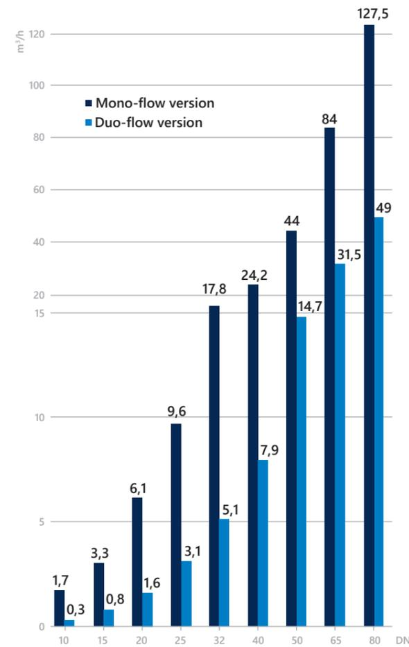
At maximum flow rate, the pressure loss is approx. 1 bar.
