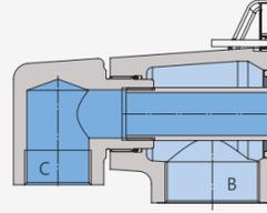
Housing connection B radial - Housing connection C radial
