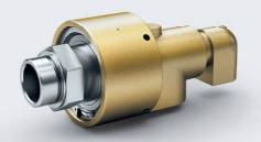
All-purpose rotary joints for water and thermal oil with balanced mechanical seal and roller bearings. Various sealing combinations are available, depending on application. Meet the special requirements of the printing and plastic industries.
