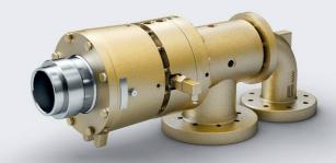
Rotary joints for hot water and steam at high pressures and speeds. Balanced mechanical seal with external water cooling. Meet the special requirements of paper and nonwoven calenders, fiber and corrugated paper plants. Suitable for big, steam-heated dryers. Patented system.
