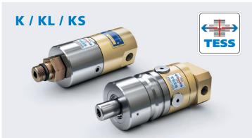
High performance rotary joints for the internal supply of cooling agent to machine tools. Series K with TESS technology (Thermal Expansion Sealing System) is substantially suitable for dry run (does not apply to KS). They can be used with a minimum amount of lubricant (MQL). This is achieved by an internationally patented proprietary development.
