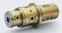
Rotary joints for compressed air. Several channels for different pressures as well as for large and small volumes. Design with special sealing rings and ceramic or hard material counter faces.
