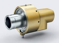
All-purpose rotary joints for water, equipped with mechanical seal and roller bearings. DXS with extremely resistant, ceramic-coated sealing face for higher temperatures and speeds and a long service life.
