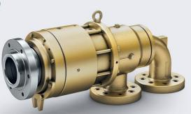
Rotary joints for thermal oil with vast temperature and speed ranges and balanced mechanical seal. DQ, DQT, DQTX with additional cooling circuit for cooling and lubricating bearings and seal. Meet the requirements of high-speed calenders. Patented system.
