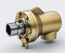
All-purpose rotary joints with maintenance-free slide bushing and sealing ring of artificial carbon. Metal-impregnated sealing ring for thermal oil; suitable for a high compressive load when used with hot water and steam. H3 with integrated vacuum valve for steam cylinders. Great number of different designs.
