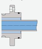
**0** K flange (loose flange) with flat packing
